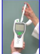
Step 3 Place tube in luminometer Results: Relative Light Units
