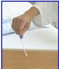
Step 1 Use special swab to sample surface
